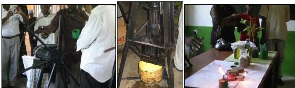
Figure 43. 'bicycle wheel' seed cracker, hydraulic piston press and akiba lamp burning jatropha straight vegetable oil (compared with current kerosene lamp) in Muhaka 2010.
