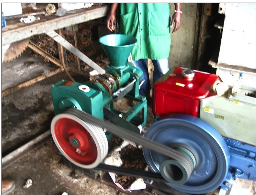
The DEGJSP press crushing Jatropha curcas L at Rea Vipingo, Kilifi 2011
