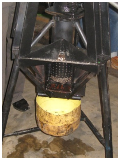
Figure 6: Small hydraulic piston press producing oil and briquettes and a Chinese manufactured diesel powered press producing oil and cake.
