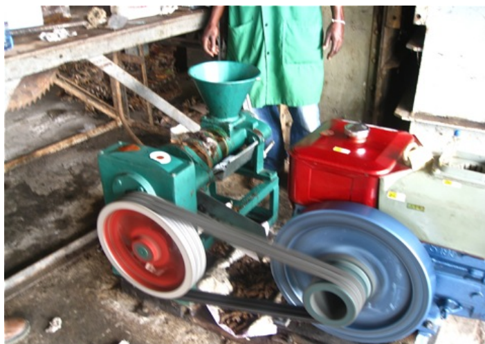
Figure 6: Small hydraulic piston press producing oil and briquettes and a Chinese manufactured diesel powered press producing oil and cake.
